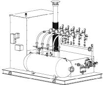
All WB/HVS systems monitor the gas pressure in the surge tank, using a pressure transmitter that is connected to a Siemens or Allen-Bradley PLC. The PLC, which is shared with the vaporizer, sequences the Venturi lines and controls all mixer safety functions. The PLC also communicates with a color LCD display with Touch Screen Operator Interface, displaying system pressures, and any trouble conditions that may occur.
