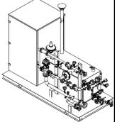
All WB/POM systems share the control panel between the WB vaporizer and the POM blender. The standard PLC is a Siemens S7-1200, or an Allen-Bradley MicroLogix-1400. All PLCs have a built-in Ethernet Interface for remote monitoring and control, and communicate with an Electronic Operator Interface (EOI) with high-resolution color LCD display and Touch Screen. Electrical connections between the POM blender and the control panel are made in two different ways:
