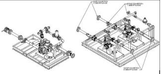
Duplex Pump Systems are manufactured as two single pumps. Except for the common skid, they do not share any essential components (mechanical independence = maximum redundancy). The pumps in duplex pump systems can be used in any combination: Pump 1, Pump 2, or Pump 1 and Pump 2 together.
