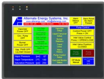
Standard EOI for Siemens S7-1200, Siemens S7-200, or Allen-Bradley MicroLogix-1400: 7-inch high-resolution (800x480) display with first-out monitor (Alarm History) 96-hour graphic TrendLine recording, trend data recording on standard SD card and remote access for monitoring and control via VNC Server / Ethernet. (unlimited client software license included).
