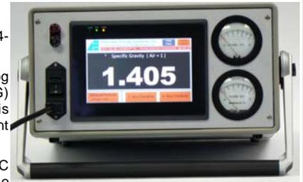
In “Detect LPG Type”, the instrument measures “raw” LPG vapor and displays the Propane/Butane ratio of the LPG.
