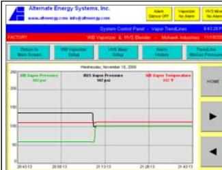
Typical Graphic TrendLine screen. This particular screen shows recorded data for vapor pressure at the outlet of the vaporizer, vapor pressure at the inlet of the mixer, and vapor temperature at the outlet of the vaporizer.
