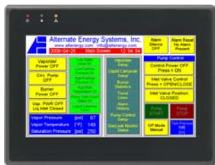
Standard EOI for Siemens PLC S7-1200 or S7-200, optional for Allen-Bradley PLC MicroLogix-1100: 7-inch high-resolution (800x480) display with first-out monitor (Alarm History) and 30-hour graphic TrendLine recording.
