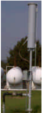
Typical Test Flare with Automatic Ignition and Weather Cap
