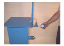
Install a UL listed shutoff valve, with a minimum rating of 250 psi gas pressure. Either a globe valve or a ball valve may be used.
