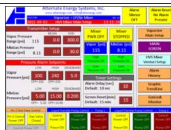
Typical Mixer Setup Screen with ranges settings for the transmitters, setpoints for low and high alarms, and Mixer Alarm Delay.
