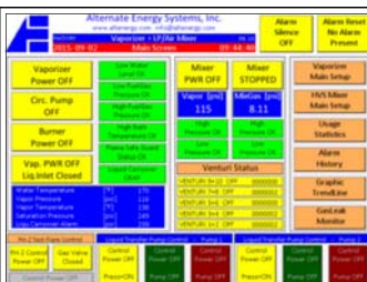
Main Screen of a typical color LCD display with touchscreen operator interface.
