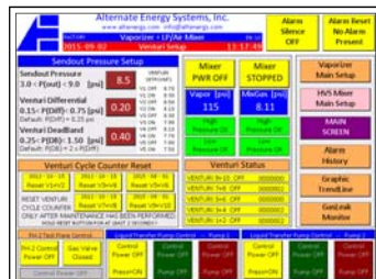
This is a typical "Sendout Pressure Setup" screen. Operators with sufficient login credentials can set the sendout pressure and the ON/OFF pressures for the Venturi banks through simple touch screen inputs in the dark-red colored fields.
